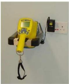
Regulations for Radiation Protection Ordinance require that anyone working with unsealed radioactive materials must be checked regularly to see whether work areas, protective clothing or the body surface has become contaminated
