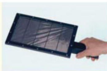
Fig. 2: Large-area, thin-layer plastic scintillation detector
