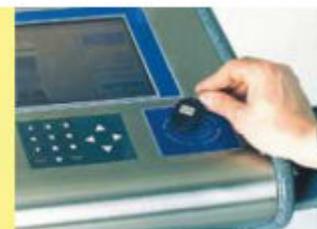
Fig. 3: Transponder for person related measurement
