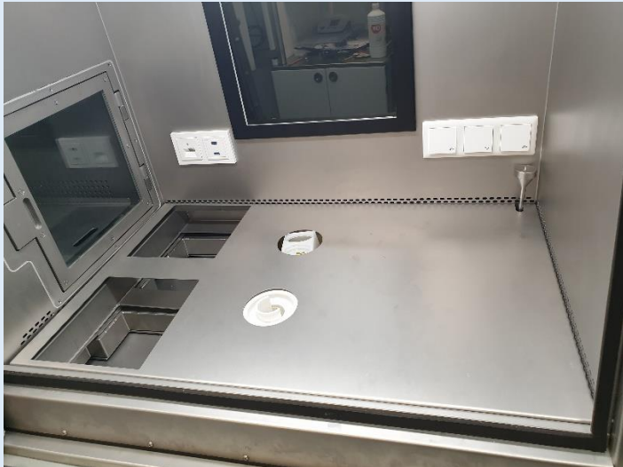
Inside position of Gallium drawers left - waste & dose calibrator in the middle and right corner the permanent particle counting Class A measurement.
