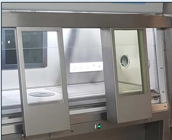
Double moveable lead glass. The right of has 30mm Pb equivalent
