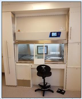
**Most sold working example**: left side pharmacy cabinet for placing disposables/printer etc.. The workspace in the middle for 2 Tc-Generators, 1 x ionisation chamber and 1 x waste bin and on the right side even the big 2 x 60 litres waste containers.
