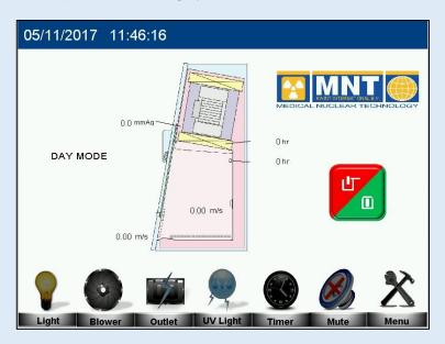
Touchscreen (frontside panel of the cabinet) does not only show all commands like any filter obstruction, speed limits, technical problems, lifting Tc-generators, but can also be supplied in many languages.
