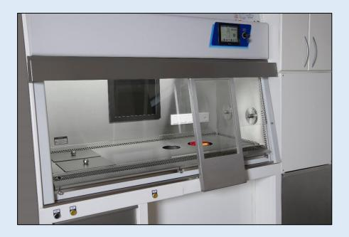
Cabinet can be supplied in many different solutions but quite a standard one is on the left side housing for 2 Tc-Generators, in the middle a built in dose calibrator with monitor on the back, a 2 litre needle waste basket, and on the right side wall a unit to be connected with 2 x 60 litre waste separation unit
